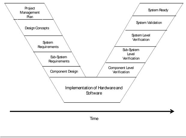
While this model may not precisely match the design process for any single designer, it does represent the generic steps that should be followed when dealing with the design of an integrated system. The advantage of understanding the design process in a generic manner is that key milestone dates can be identified. Once the key milestone dates are determined, it is then possible to identify the timing of Concurrent Engineering activities to ensure reliability requirements are being addressed.
